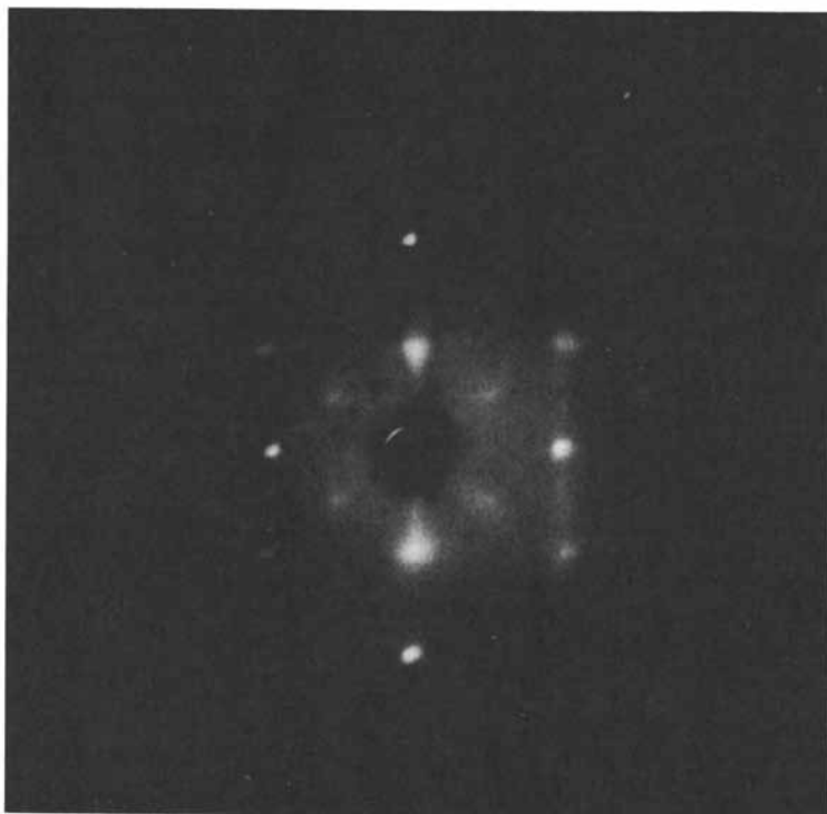
Figure 5. LEED pattern resulting from immersion of a \text{Cu}(110)c(2 \times 2)-\text{Cl} structure into water. \text{Cu}(110)c(4 \times 2)-\text{Cl}_2\text{O} pattern, 61 eV.
