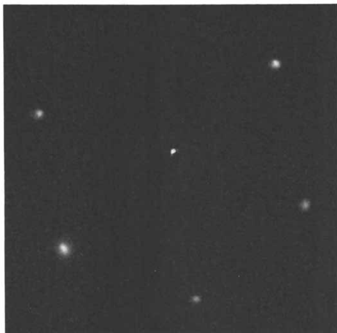
Figure 3. LEED pattern of the Pt(111) electrode used for the reported research. The beam energy was 65 eV.
